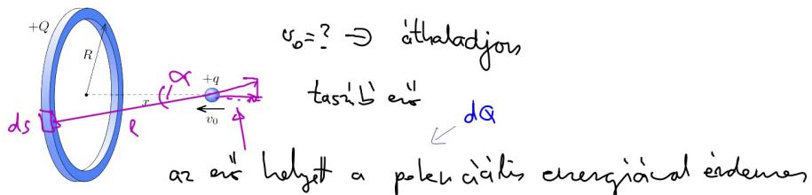
$$q d\varphi(x) = \underbrace{\frac{qQ}{2R\pi} \cdot ds \cdot \frac{1}{l(x)}}_{dQ} \quad l(x) = \sqrt{x^2 + R^2}$$
